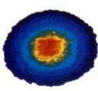
The effects of beam smoothing are dramatically evident in these cross-sectional images of a laser beam: left, without smoothing; right, with smoothing (J. Knauer, University of Rochester). Without smoothing, the laser beam can seed and then drive the Rayleigh-Taylor instability, which, for fusion capsules, would thwart adequate fuel compression.
